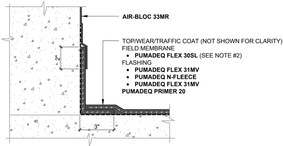
**AIR BARRIER INSTALLED AFTER PUMADEC SYSTEM**
