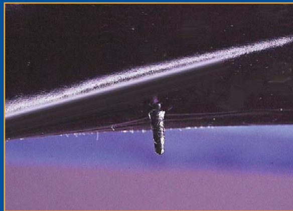
Self-sealing around nails or screws
